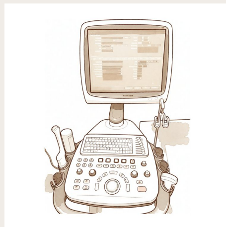
An ultrasound machine: a hand-held probe sends and listens for sound waves, building the picture live on the screen.
