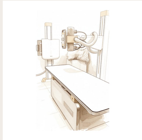
An X-ray machine: a tube above the table sends a brief beam through the body to a detector beneath it. Nahid.rajb / Wikimedia Commons, CC BY-SA 4.0
